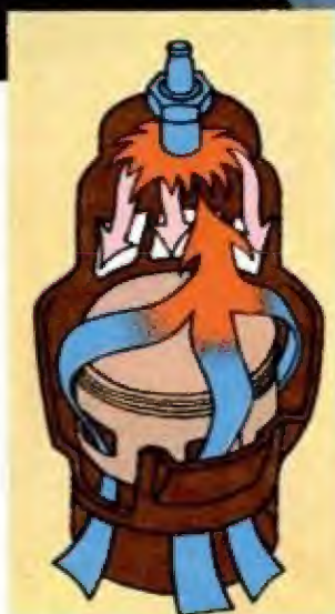
Johnson's Loop-Charged design incorporates flat-top, lighter pistons. Less weight, less stress, runs cooler. Result: More performance.
